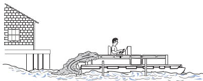
Blockage of boat exhaust by obstruction
